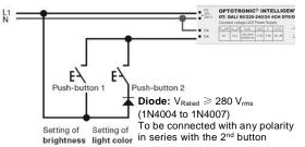
This driver supports single and double button Touch DIM operation. The 2<sup>nd</sup> button must be connected in parallel with the 1<sup>st</sup> by means of a diode.
