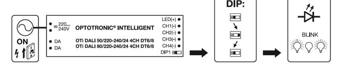
For instance, in order to reconfigure the driver for a new DT6 load configuration, after connecting or disconnecting new loads, move the dip-switch from ON to OFF, then from OFF to ON, during power-on or powering on after each operation.
