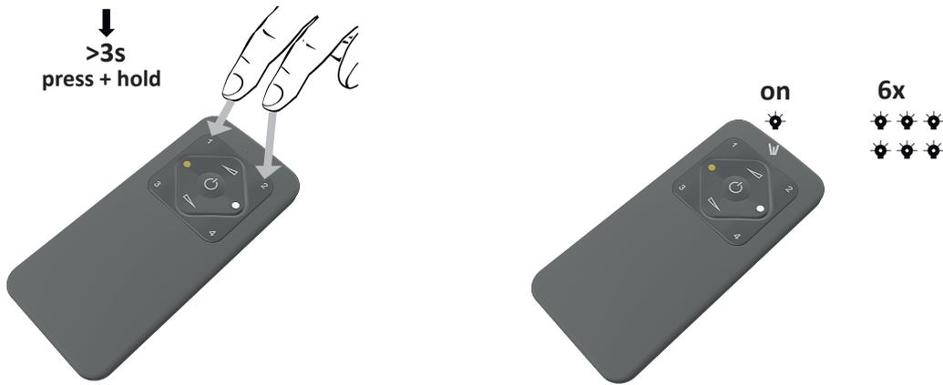
The successful start is confirmed by a fast flashing of the red indicator LED. If the connection is successful, the red LED flashes 6 times. The successful connection is also confirmed by the flashing of the connected LED light
